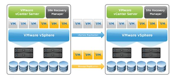
FIGURE 16 - vSphere SRM Architecture
