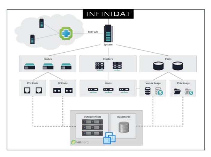
FIGURE 21 - InfiniBox Management Pack for VMware vRealize Operations
