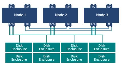
IMAGE 2 InfiniBox front-end and back-end connectivity
